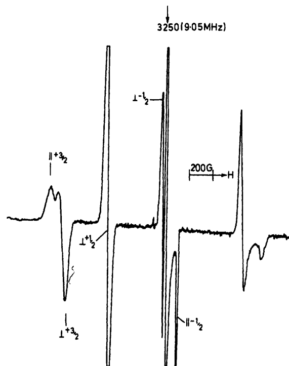
FIGURE 7 First derivative X-band e.s.r. spectrum for \text{Ph}_3\text{AsO} in \text{CD}_3\text{OD} , at 77 K, after exposure to ^{60}\text{Co} \gamma -rays, showing features assigned to \text{Ph}_3\text{AsO}^- or \text{Ph}_3\text{AsOD} radicals
